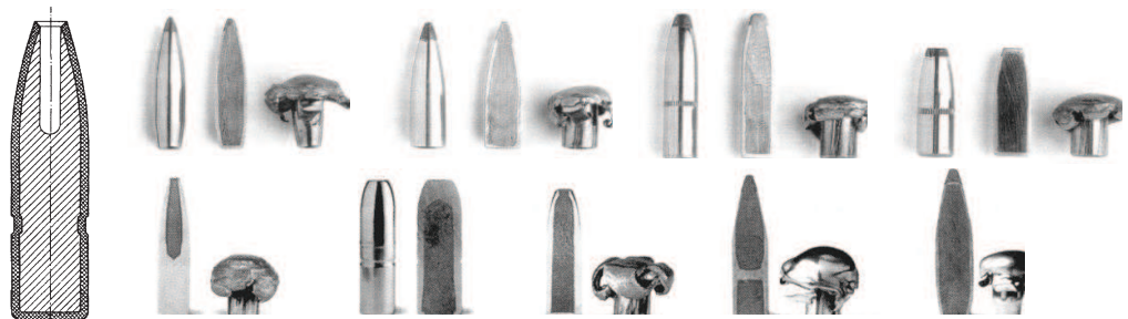
Figure 3 - The mushroom deformation of a bullet tip
