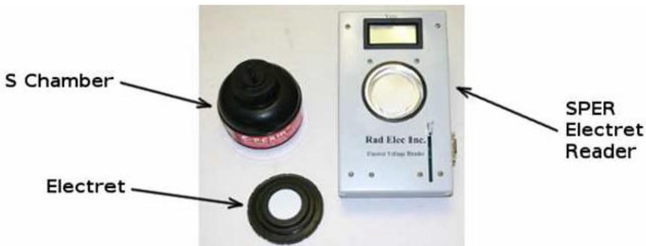
Figure 1. The E-PERM® Electrets system
