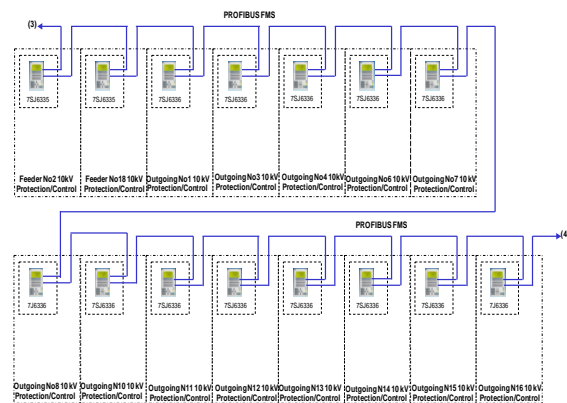
Fig. 7 10 kV protection and control cubicles
