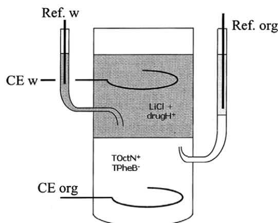
Fig. 2. Schematic representation of the electrochemical cell used in the experiments. The aqueous (w) phase contained LiCl and the protonated form of the drug under study (DrugH<sup>+</sup>), and the organic (org) phase contained tetraoctylammonium tetraphenylborate salt (TOctN<sup>+</sup> TPheB<sup>-</sup>). CE, counter electrodes; Ref., reference electrodes.
