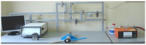
Figure 2. Apparatus for high presssure density measurements
