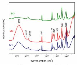
Fig. 1. FTIR spectra of three membranes prepared using the same polymer mixture but different coagulation mixtures
