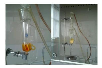
Figure 2. Soxlet aparatus for extraction
