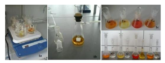
Figure 1. Phases of vacuum filtration method for extracting the oleoresins (1a maceration; 1b vacuum filtration; 1c and1d dilution of oleoresins)
