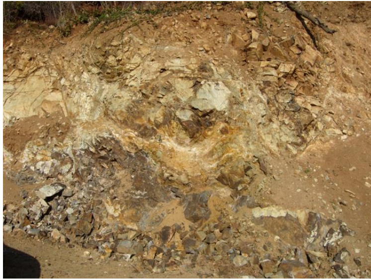
Figure 3: Fresh gabbro covered with altered gabbro with poor physical-mechanical characteristics
