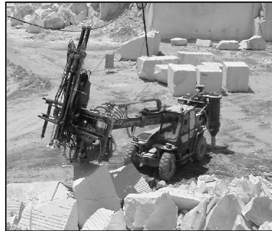
Figure 5. Drilling machine Perfora , tipe "Handu maxdrill hm02" in the open pit quarry "Sivec"
