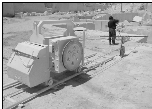
Figure 6. Diamonds wires saw machine tipe ALFA 840, Benettimachines , Verona, Italy
