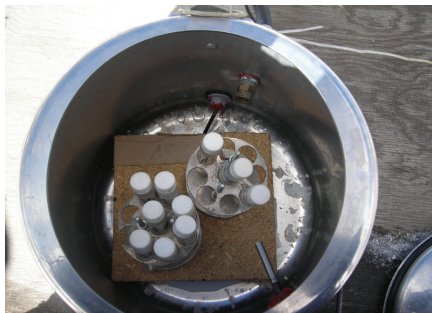
Figure 2. Positioning of bubble dosimeters inside the pressurized box, as used at Chacaltaya.
