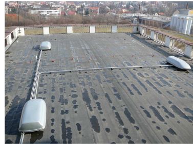
Figure 1: Typical ALTA/CZELTA detection site: The three stations shown house scintillating detectors
