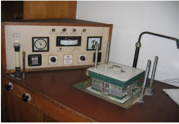
Fig. 2- D-r "BOK" instrument used to measure thermal characteristics
