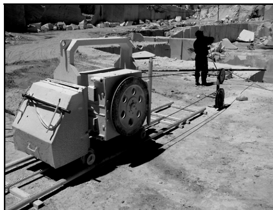
Figure 3 Preparation of cuts for "V" profile with diamond wire saw
