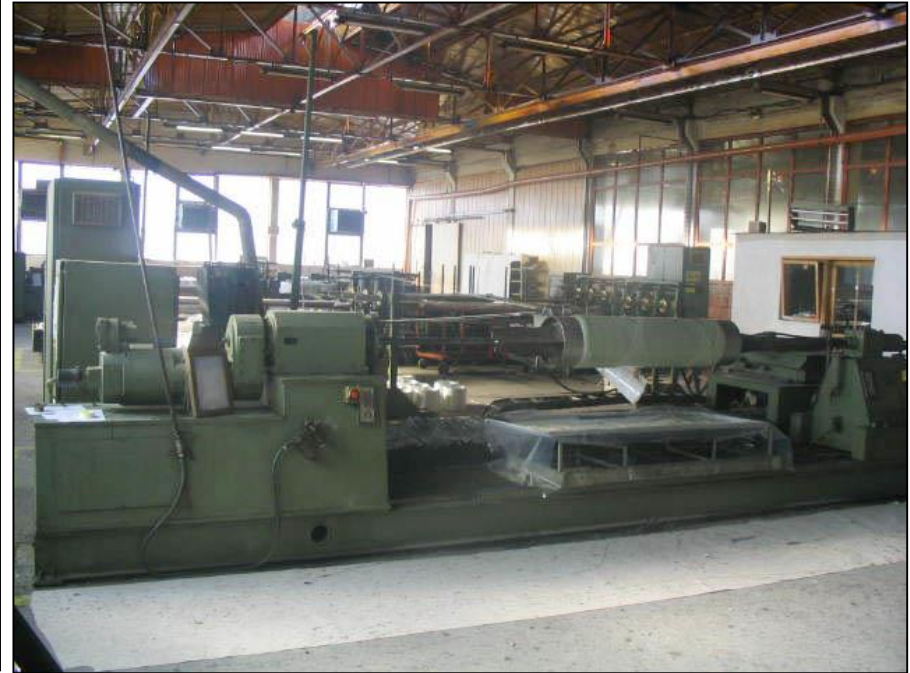
Multi axes computer controlled winding
