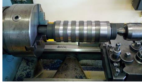
Figure 2. Special set up for exploring the characteristics of the surface layer during turning.
