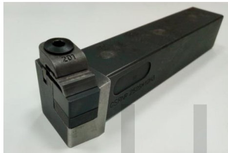
Figure 3. a) The CSRNR 25x25 M12H3 cutting board holder from HERTEL, b) Cut-off inserts SNGN 120708-120712-120716 from mixed ceramics MC 2 ( \text{Al}_2\text{O}_3 + \text{TiC} ) from the company HERTEL
