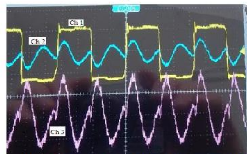
f_s = 0,5 f_0 = 2\,979 Hz, Ch1=50V/div, Ch2=100A/div, Ch3= 2000W/div, time=80μS
