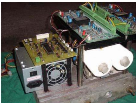
Fig. 6. The control module with IGBT drivers and IGBTtransistors.
