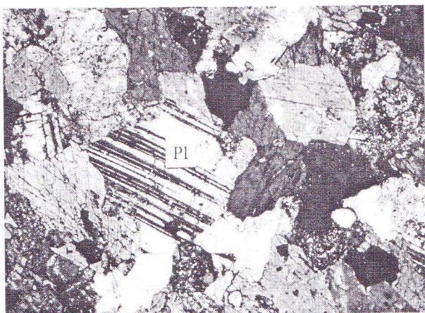
Fig. 7. Microphotograph of plagioclases in medium size-grained amphibole gabbro of Novo Selo – Kriva Lakavica shown, X N, magnification 6.3. Note: Pl – plagioclase
