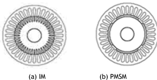
Figure 1. Cross-section of analysed motors
