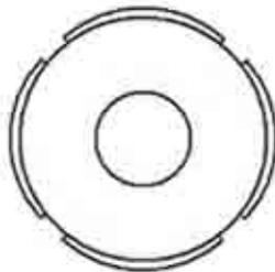
Figure 4. Rotor configuration of IPMSM
