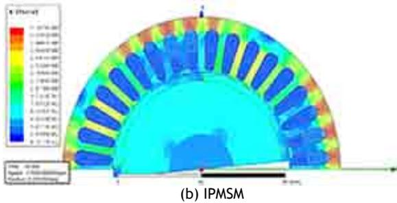
Figure 6. Magnetic flux density at motor cross-section
