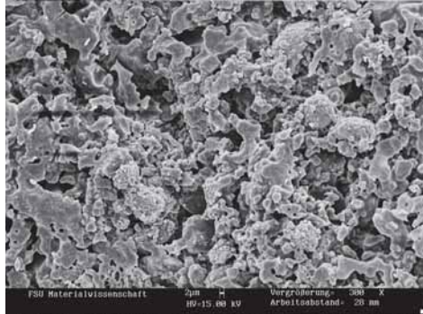
Figure 14. Microstructure of TFA-MA30 sintered at 1130 0 C/1h, (bar 2 µm)
