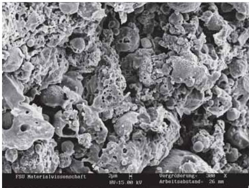
Figure 10. Microstructure of TFA compacts sintered at 1150°C (bar: 2µm)
