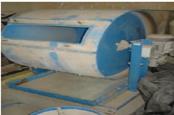
Figure 14: 28 inch (700mm) diameter tumbler
