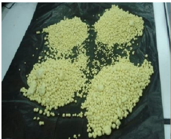
Figure 11: Sample quartering method
