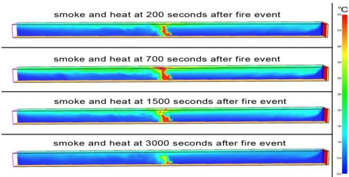
Fig. 14. CFD simulation of fire scenario 1, in computer program PyroSim
