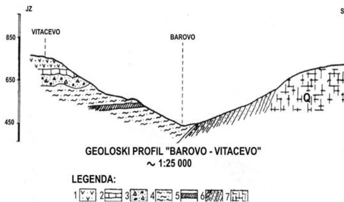
Fig. 6 Geological cross-section of Barovo-Vitacevo (Boev, 1988) 1. Conglomerate tuff; 2. Lacustrine deposited tuff; 3. Lacustrine deposited tuff with epiclaste larger than 2 mm but smaller than 64 mm in size; 4. Neogene lacustrine sediments; 5. Tuffs; 6. Eocene marls; 7. Quartzites
