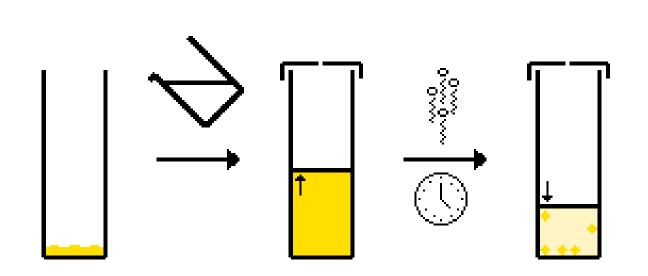
Single crystals with quality for structure determination were obtained by slow controlled rate of solvent evaporation techniques.
