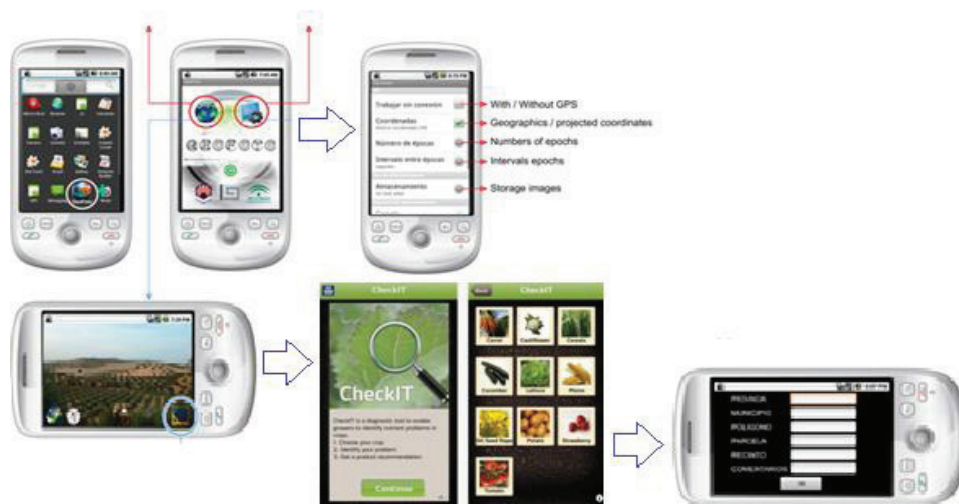
Fig. 1 GeoFoto screenshots: (a) access to the application, (b) initial screen accessed by the user (c) settings menu, (d) main menu and (f) digital blackboard, (e) possible application in the identification of pests and diseases
