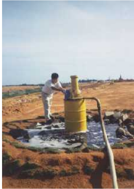
71. (Ampang Jajar Landfill, Malaysia) Figure 71. Example of circulation of leachate (Ampang Jajar Landfill, Malaysia)
