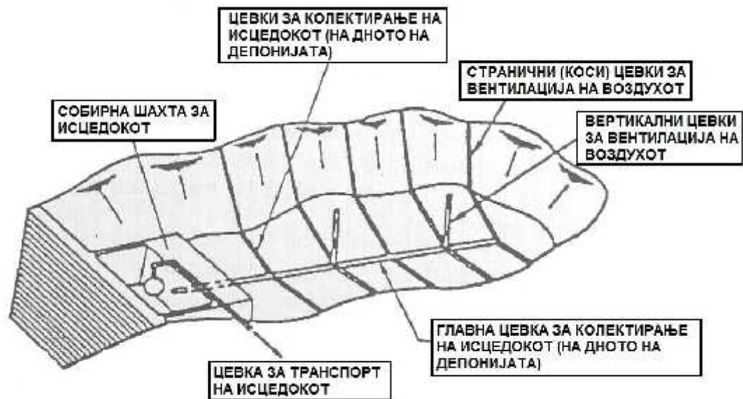
Figure 26. Construction of leachate collection pipes and gas venting pipes with retention pit inside landfill
