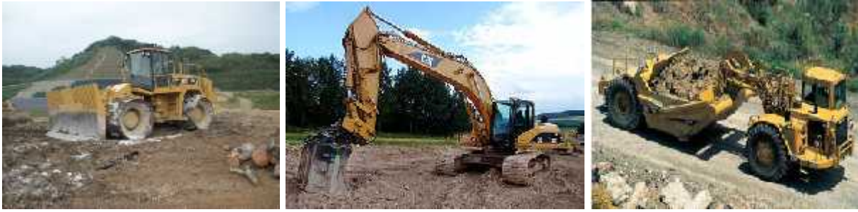
( , , ) Figure 82. Machinery required for the sanitary landfill (Bulldozer, Compactor, Dredge and Scraper)
