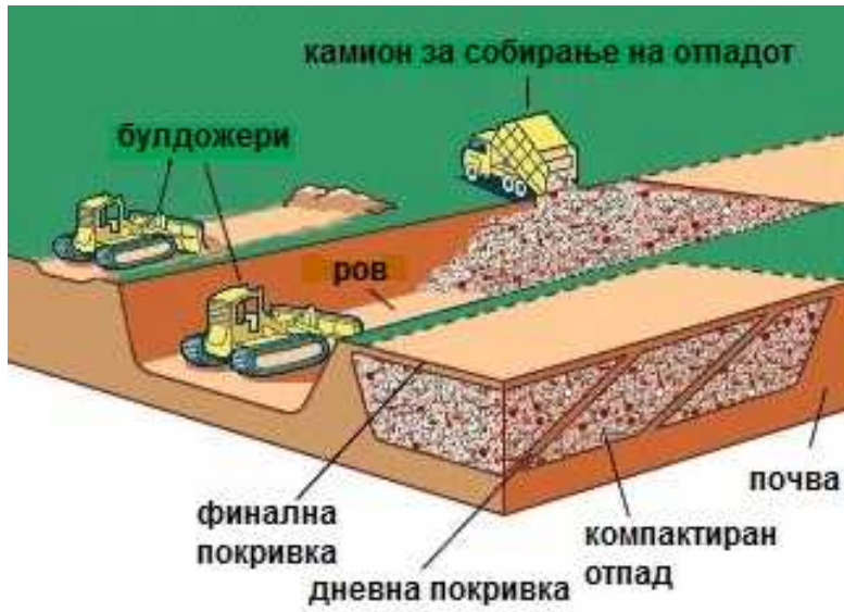
77. Figure 77. Trench Method
