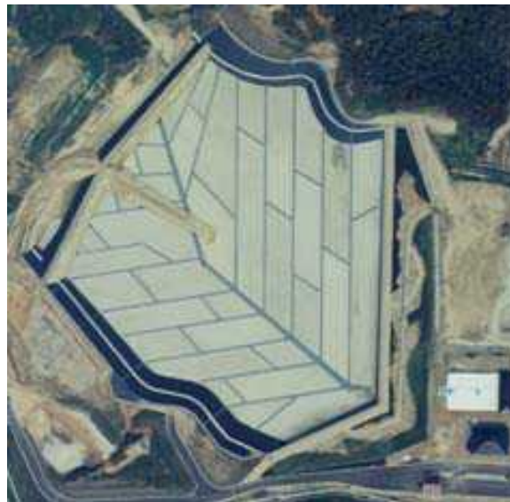
Figure 38. Placement example of leachate collection discharge pipes (Nakata landfill, Fukuoka-Japan)
