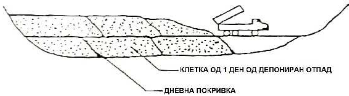
80. Figure 80. Cell Method
