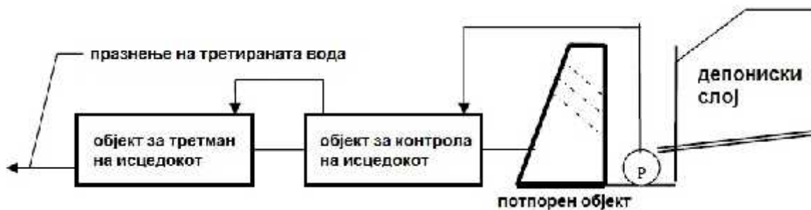
30. ( ) Figure 30. Method of pit-pump (in-side) of leachate
