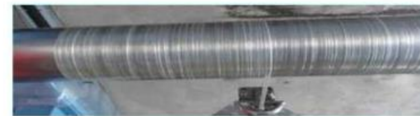
Hoop winding ( \theta = 90^\circ )
