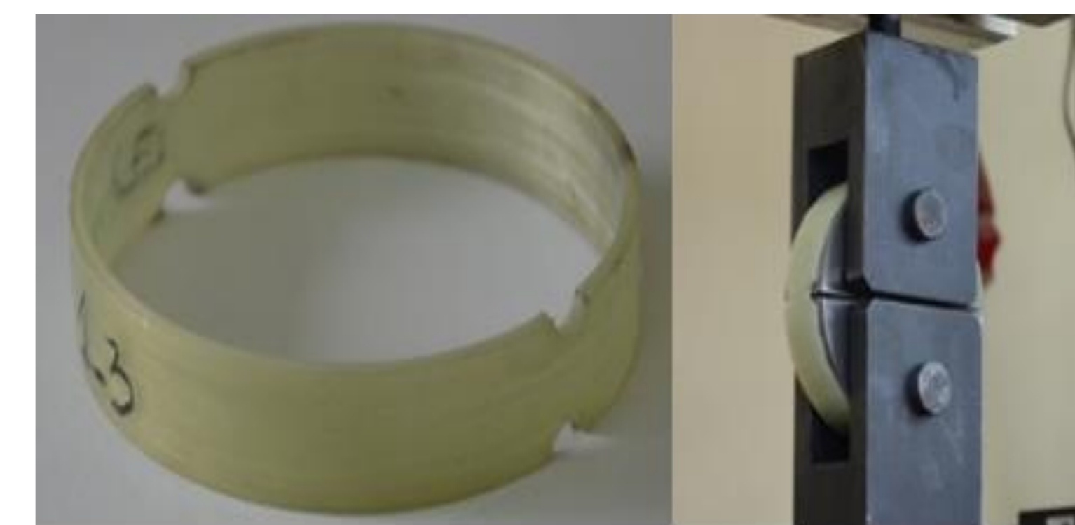
Figure 4. Split-disk test specimen and test fixture with specimen for hoop tensile testing
