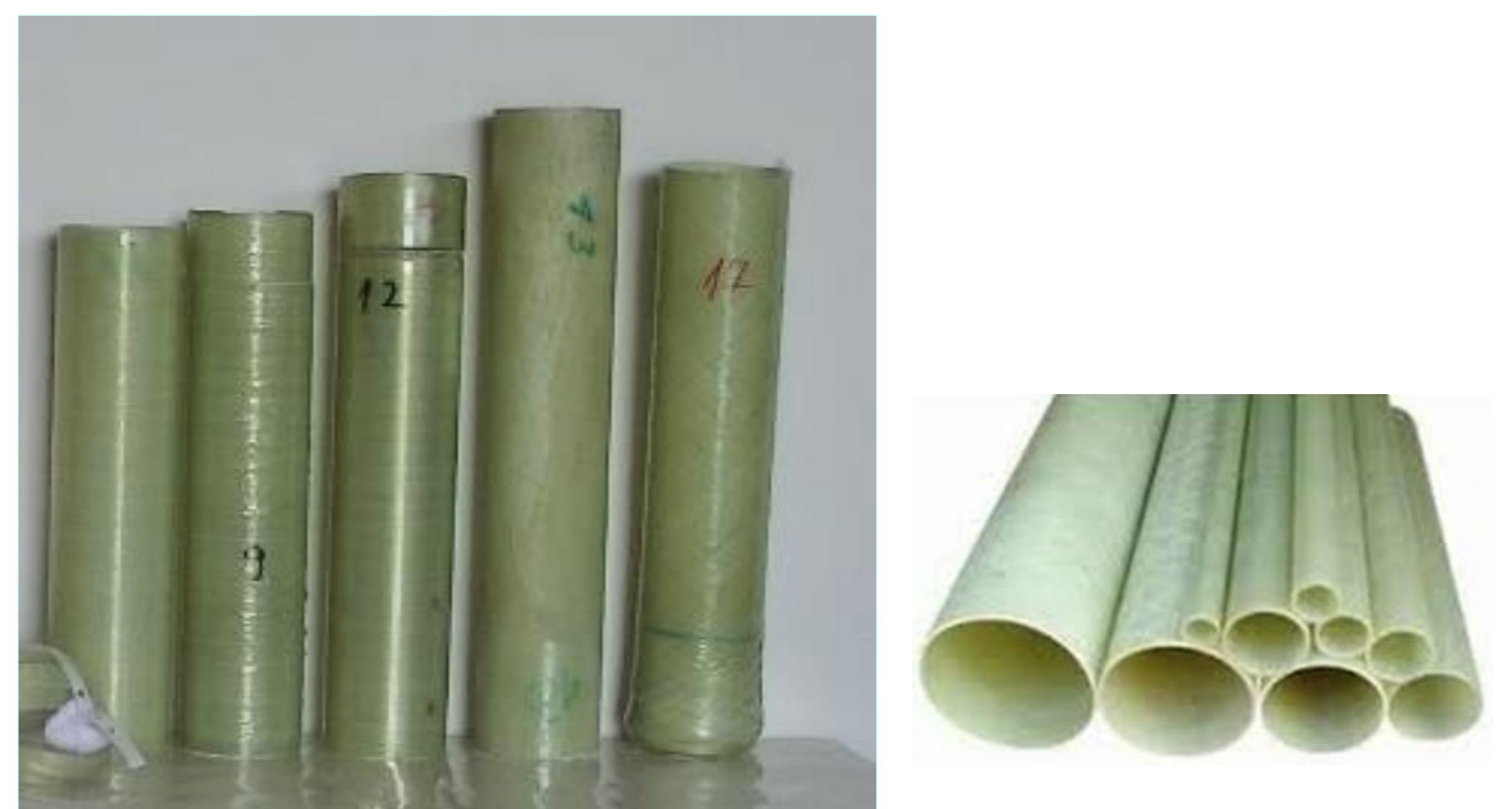
Figure 4. Produced glass fiber/epoxy resin filament wound composite pipes
