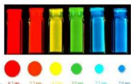
Fig. 1. CdSe QDs with size range of 2 to 6.5 nm, with decreasing crystal size the band gap of the crystal increases and the dot gives off more energetic or blue photons
