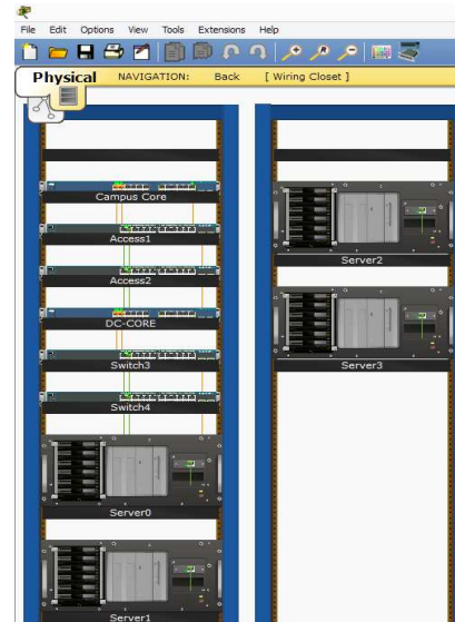
Figure 6. The physical workspace (Wiring Closet) with graphical view of network devices and connections
