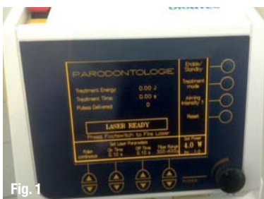
Fig. 1 The Ceralas D15/810 nm diode laser. Fig. 2 Gingival display before laser treatment. Fig. 3 Abnormal growth of the gingival tissue around the central and lateral incisors and the canines in the maxillae.
