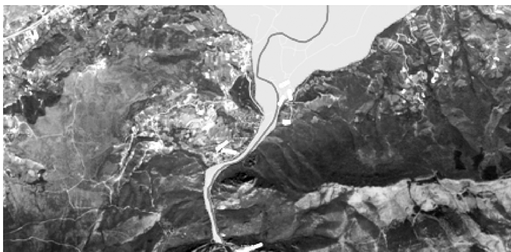
Figure 13. Flooded area from eventual demolishing of the dam “Matka”
