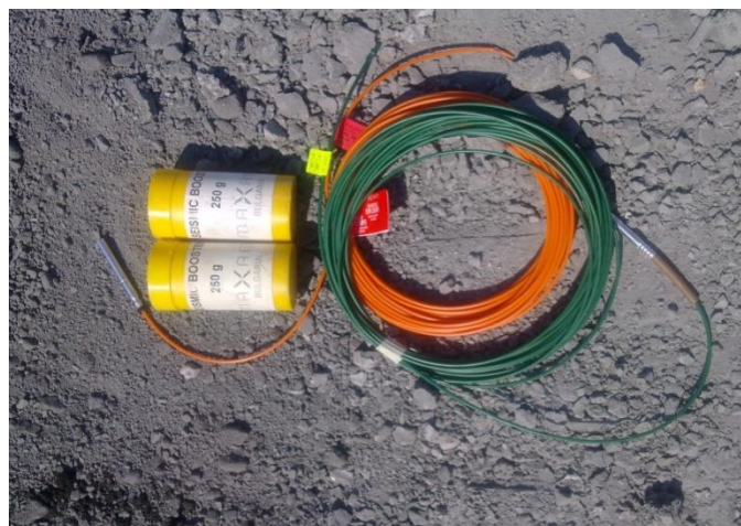
Figure 3. Non-electric detonators 300 and 500 ms with TNT boosters
