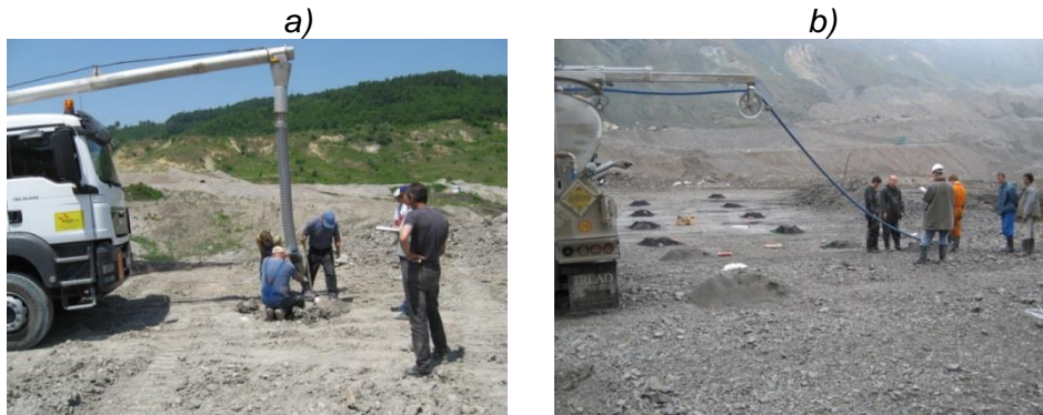
Figure 5. Mechanized charging with: a) ANFO explosive and b) EMULSION explosive
