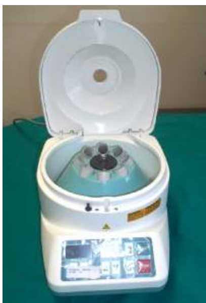
Figure 1 Centrifugal machine for the Platelet Rich Fibrin (PRF) at Department of Oral Surgery, Faculty of Dentistry University of Sarajevo
