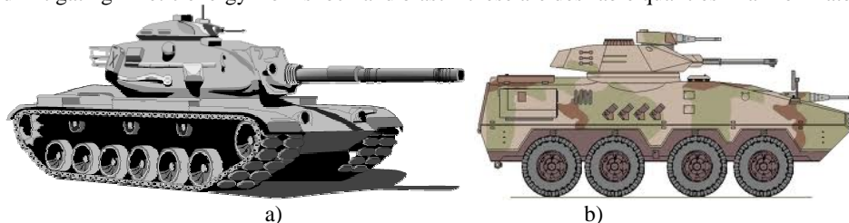
Fig. 1. a). RHA and CHA has been used in tanks since World War II such as in the M60 Patton tank, b) Light armored vehicle is partly composed of HHA
